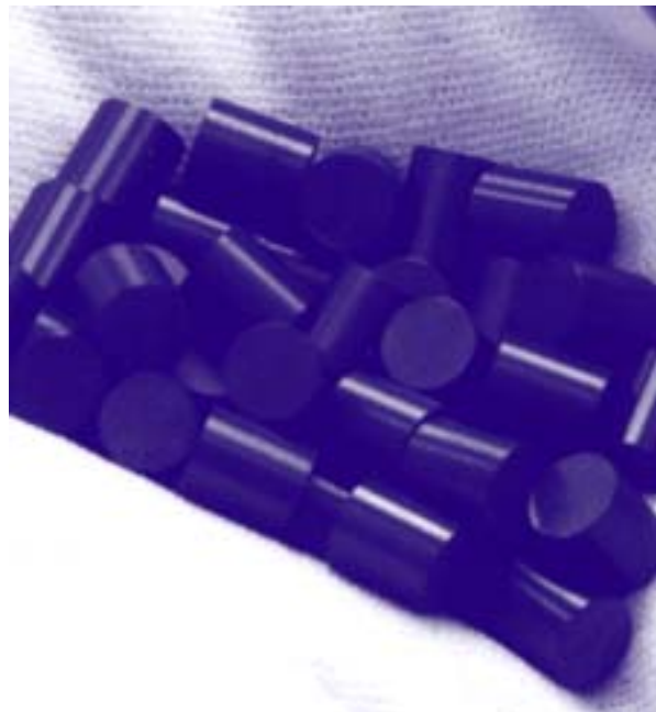
Solid ceramic nuclear fuel pellets, each slightly larger than a pencil eraser, containing both uranium-235 and uranium-238.
