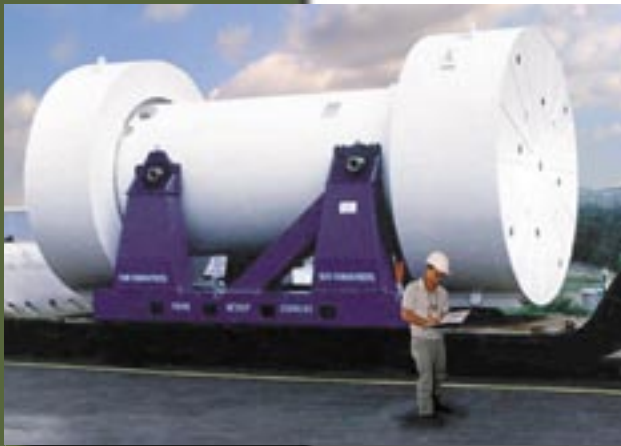
Rail cask with impact limiters designed for the transportation of spent nuclear fuel and high-level radioactive waste.
