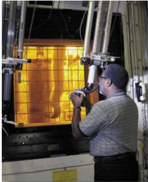
High-level radioactive waste is made solid by mixing it with glass-forming chemicals in stainless steel canisters and then subjecting it to heat. The result is a hard glass-like substance.
